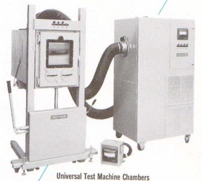
Pre-engineered standard chambers for use with most makes and models of physical testing machines. Available in a full range of high and low temperatures for performing MIL and ASTM specification tests, and for research and development. Chambers are built with temperature capabilities as wide as -300 F to +1000F. Humidity control can be added by means of the portable Humidity Servo
