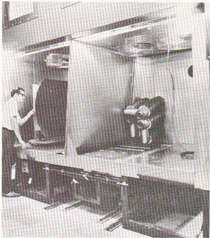
DUAL COMPARTMENTS INSIDE CHAMBER are separated by double-walled silicone-impregnated fiberglass curtain that simulates partition in aircraft between antenna section in nose and electronic equipment section.
