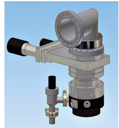
Drawing of a turbopump with roughing valve, slide valve, right angle elbow, and elbow cold trap. An optional elbow heat exchanger is shown to limit thermal face loading on the pump at high temperature.
