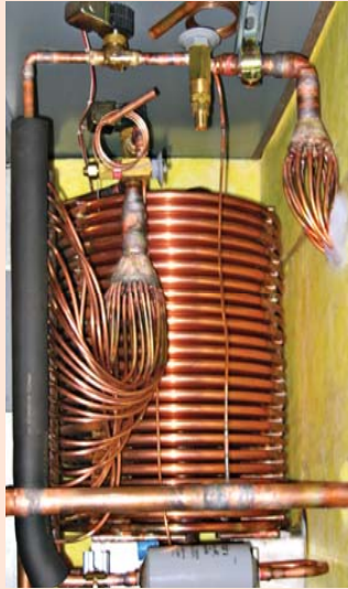
FHC Series high capacity, two compressor refrigeration system. Shown below, the Bemco exclusive, high reliability cascade heat exchanger.
