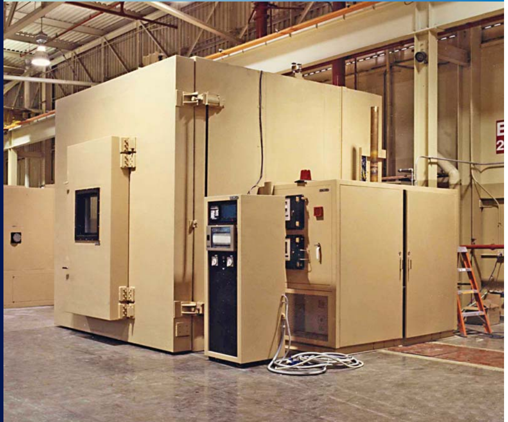
Walk-in integral (one piece welded) Temperature, Humidity, and Altitude Test Facility with man access door and full opening front door in the process of installation.
