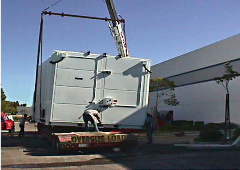
Walk-in integral (one piece welded) liquid nitrogen cooled chamber with a range of -180 C to +150 C equipped with a nitrogen atmosphere door interlock.
