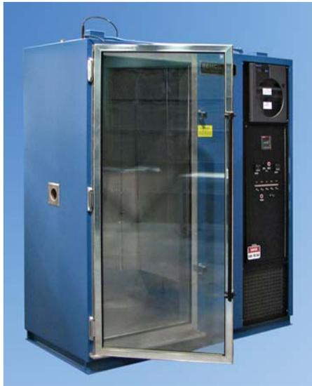
Cooling rate from 75 C to -15 C in less than 90 minutes. Heating rate -15 C to 75 C in less than 60 minutes. Both with the chamber empty.
