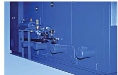
Bemco KDR4-20/65C fan motors and a water cooled condenser extend from the rear of the chamber and add approximately 12-inches to overall depth.
