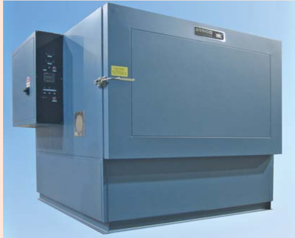
Larger and custom sizes are available. A custom LDF67 is shown with interior workspace dimensions of 37" high by 62" wide by 51" deep.
